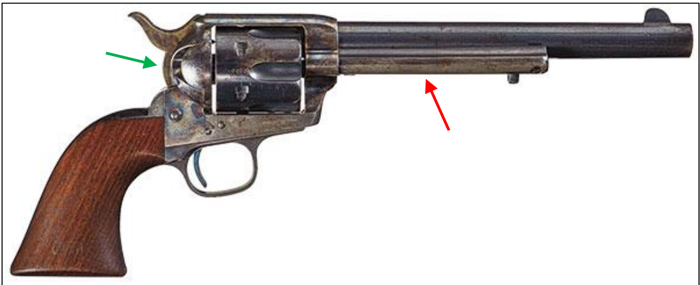
Figure 1. The Colt Single Action Army Revolver. The Colt revolver required the user to eject and load one chamber at a time, as they rotated the cylinder to line each chamber up with the side-mounted loading gate. The green arrow points to the loading gate, the red arrow points to the ejector.
