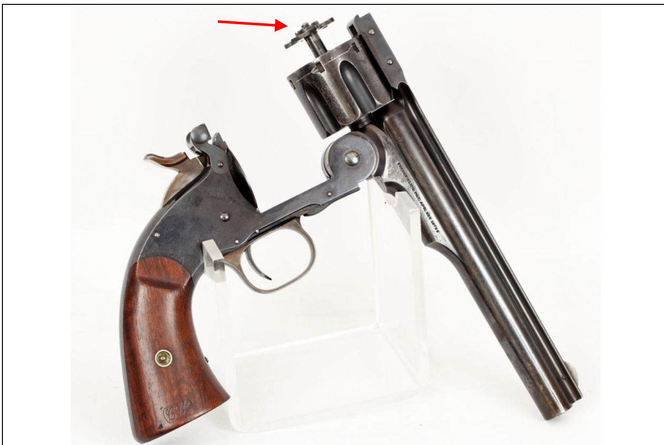
Figure 3. The Smith & Wesson Schofield is considered a “top break” revolver. The arrow points to the ejector. Top-break revolvers had the ability to eject all empty shells simultaneously, and exposed all chambers for reloading.
